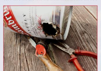
inwards with pliers for increased safety. The edge must be round so as not to cut through the LED cable. For increased safety, wrap the hole with electrical tape.
