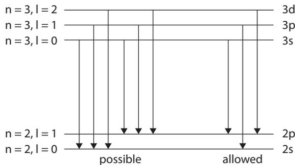
**Figure 1.3:** Transitions from orbital  $n = 3$  to orbital  $n = 2$ .
