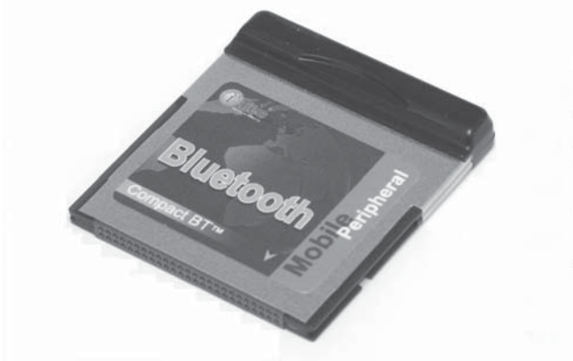
Obr. 1.6: Bluetooth modul do CF slotu
